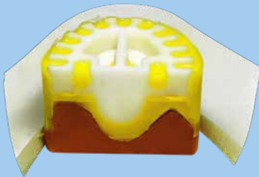
Cross-section of a flaskless duplicating mould
